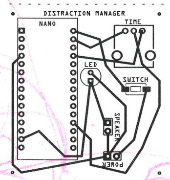
lx Arduino Nano lx 10 OHM potentiometer lx led light lx speaker 2x female header with 15 pins Ex male header with 15 pins lx switch lx power adapter 1x 9V battery or additional questions write to: isa neza herlecagmail.com
