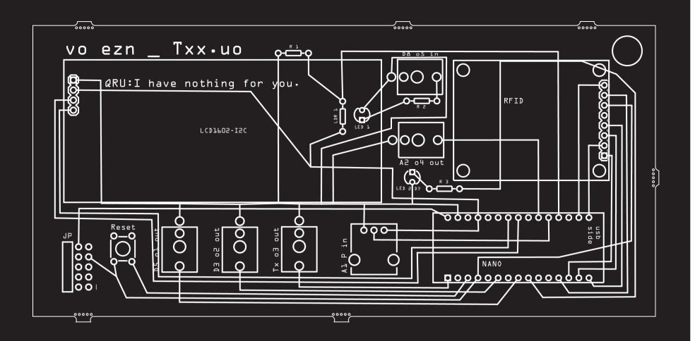
Txx.uo consolidates two contrasting radio frequency implementation modes: RFID reader scans the cards/objects containing RFID tags using radio waves and LCD screen displays a Q-code\* Einternationally established three-letter abbreviation used in radio communication].
