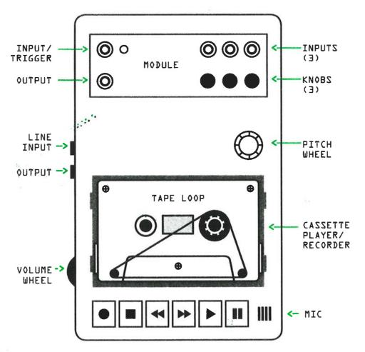
L) A DESKTOP CASSETTE PLAYER a multitrack recorder or a walkman with an amplifier. You can make a pitch control to your device by adding a potentiometer.
