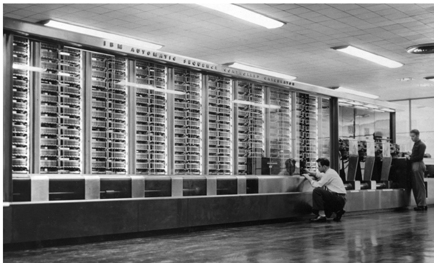
The IBM Automatic Sequence Controlled Calculator (ASCC), known as The Harvard Mark 1, was a general purpose electromechanical computer that was used during the last part of World War II. (source: Wikipedia)
