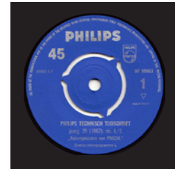
2 “Rekengeluiiden van de PASCAL” (Calculation sounds from PASCAL) is a 7” record with sounds produced by the PASCAL (Philips Akelig Snelle CALculator) from the Philips NatLab. The recordings consist of computing noises from the computer. Side A contains recordings from regular operation and mechanical noises. On the B-side is a recording of a prime number calculation. The record was included in the Philips Technical Review Vol. 24 (1962) No. 4/5.
