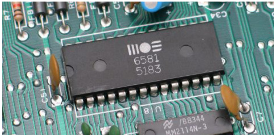
The MOS Technology 6581/8580 SID (Sound Interface Device) is the built-in programmable sound generator chip of many models of Commodore computers. It was one of the first sound chips of its kind to be included in a home computer prior to the digital sound revolution. (source: Wikipedia)
