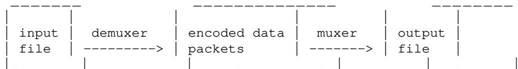
Since there is no decoding or encoding, it is very fast and there is no quality loss. However, it might not work in some cases because of many factors. Applying filters is obviously also impossible, since filters work on uncompressed data.
