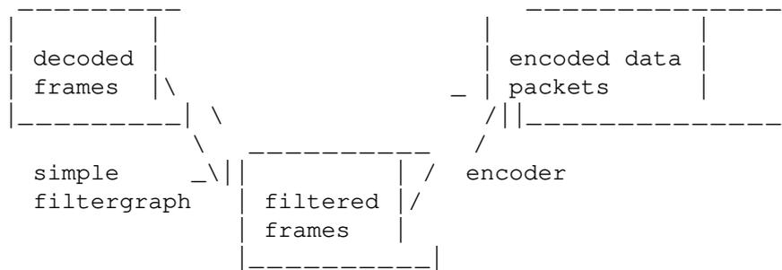
Simple filtergraphs are configured with the per-stream **-filter** option (with **-vf** and **-af** aliases for video and audio respectively). A simple filtergraph for video can look for example like this:
