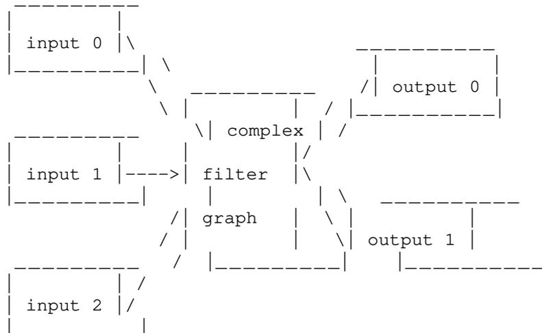
Complex filtergraphs are configured with the `-filter_complex` option. Note that this option is global, since a complex filtergraph, by its nature, cannot be unambiguously associated with a single stream or file.
